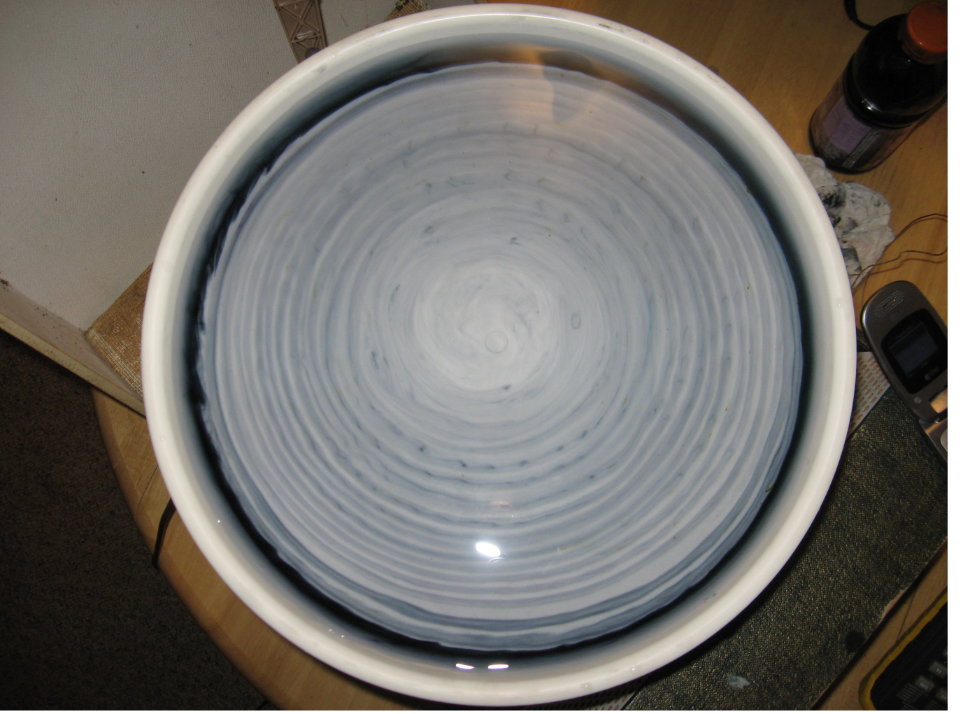
FIG. 4: Picture of the typical structure of convective rings formed during the preconditioning phase. The rings have a minimum ring diameter d_{min} , and the distance between concentric rings decreases away from the center of the dish. Rings close to the center of the dish are beginning to roll up and form vortices due to shear instability.
