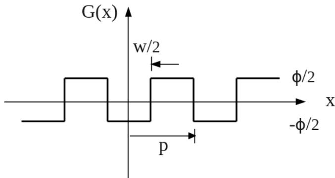
Figure 3: Functional representation, along the  $x$  direction, of a phase grating of groove width  $w$  and period  $p$  with modulation depth  $\Phi$ .
