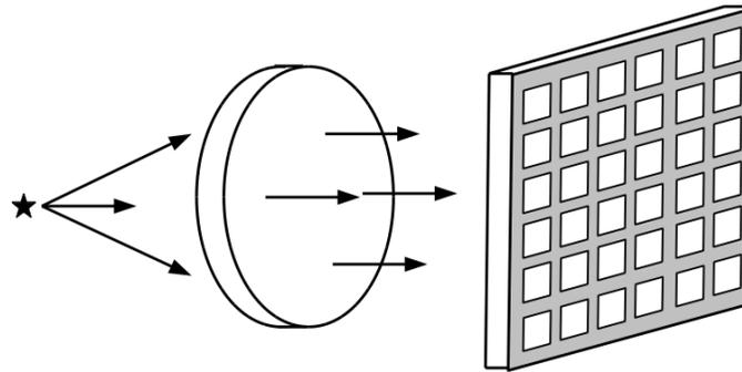
Figure 1: Three dimensional sketch of a plane wave illuminating micro lens array.
