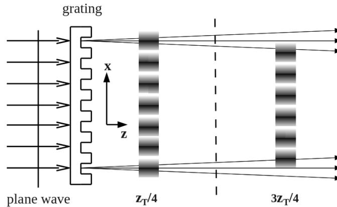
Figure 4: Two dimensional representation of a grating array illuminator in the Fresnel region, at sub-multiples distances to the Talbot length.
