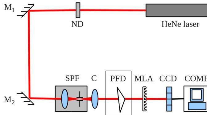
Figure 6: Schematics of the experimental setup to observe the effects of inserting an imperfection on the imaging system through the distortion of the phase front.
