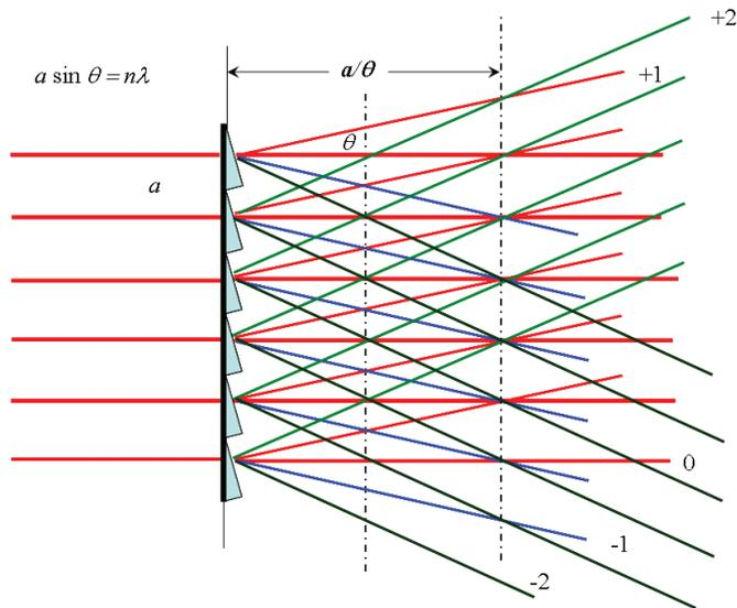
Figure 2: Ray tracing for a transmission grating.
