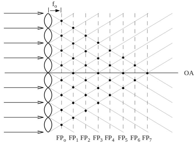
Figure 7: Ray tracing of light incident on a micro lens array of focal planes (FPs) on a 2-D representation. Each lens has a focal length  $f_0$ .
