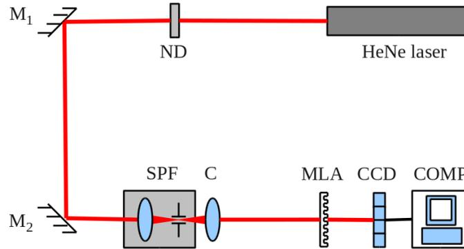
Figure 5: Schematics of the experimental setup to observe/measure the Talbot length and its sub-multiples.
