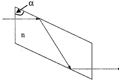
(d) In constructing a Fresnel rhomb, what restriction is imposed on the material's refractive index..
