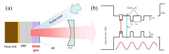
The QWs are made from GaAs and the barriers are  $Al_xGa_{1-x}As$  which is lattice matched to GaAs (i.e. no strain). Assume the operation is at room temperature (T=300K) where
