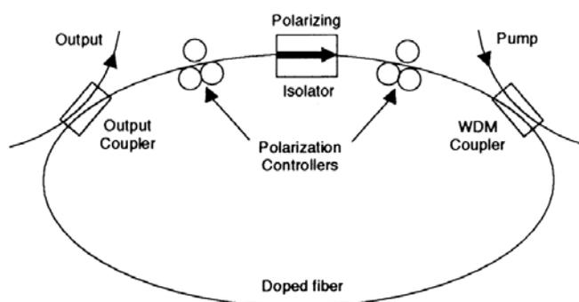
Fig. 1 Schematic design of a fiber laser passively mode locked through nonlinear polarization-rotation.
