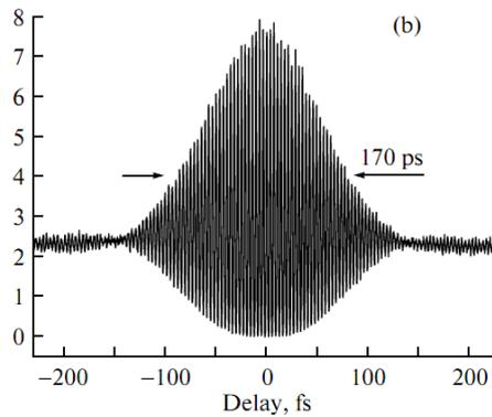
Fig. 3 Typical auto-correlation trace of the output pulses.
