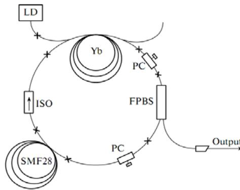
Fig.2. sketch of the fiber laser with ultra-long cavity. PC: polarization controller; ISO: isolator; LD: laser diode.
