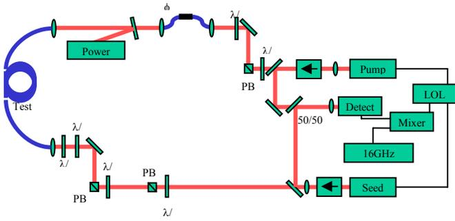
Figure 8: SBS Modulation Scheme Set-up
