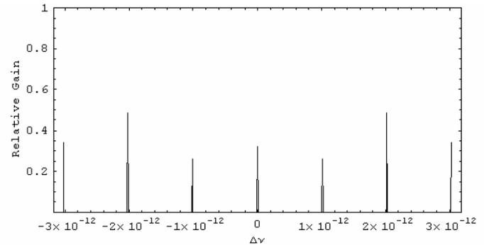
Figure 11: Relative SBS Gain due to Phase Modulation
