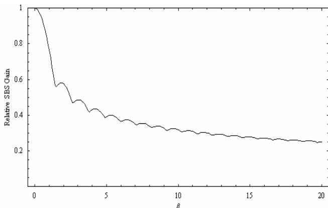
Figure 10: Model of Modulation Depth versus SBS Gain
