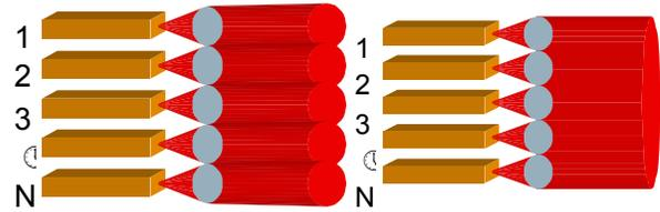
Figure 4: Non-coherent versus Coherent Beam Combining
