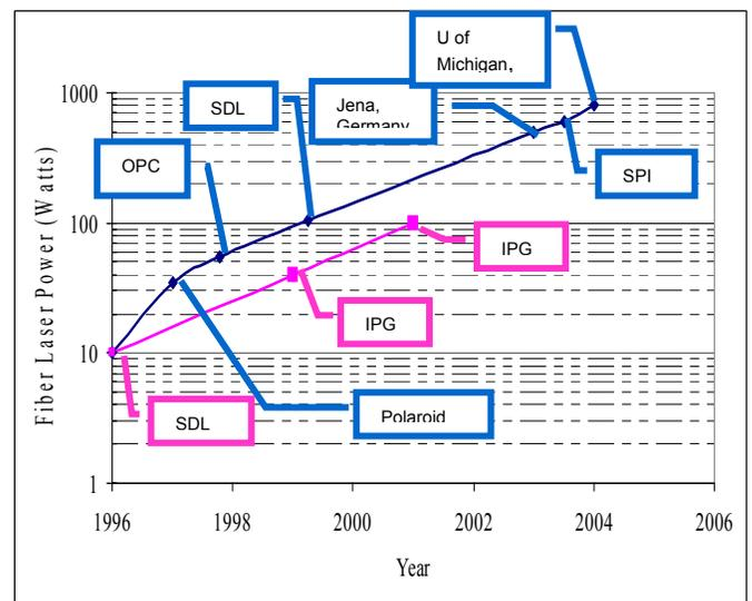
Figure 3: History of Fiber Laser Power Output
