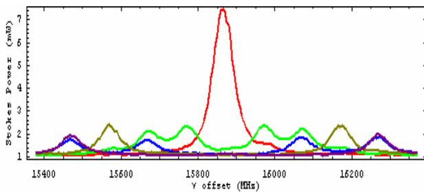
Figure 9: SBS Seed Response to Phase Modulation
