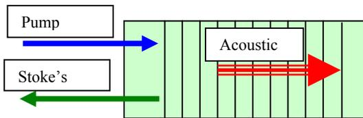
Figure 1: SBS in Single-Mode Fibers
