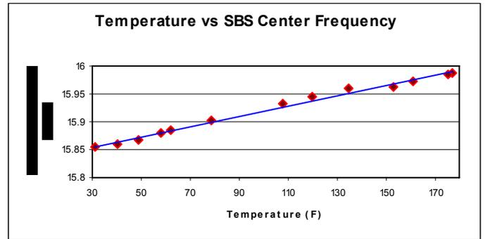
Figure 7: Effects of Temperature on Stokes Frequency
