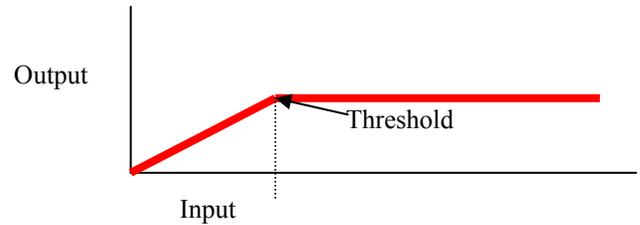
Figure 2: SBS “Clamped” Power Threshold
