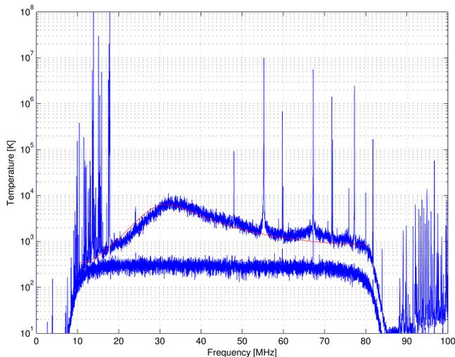
Fig. 6. *Top curve*: Spectrum acquired using an LWA prototype active antenna (similar the one shown in the right of Figure 3), with the ARX and A/D described in the text. 1 s integration. Also shown overlaying the top curve is the result predicted from a sky model. *Bottom curve*: Same measurement performed with a 100 ohm (matched) load replacing the dipole arms.
