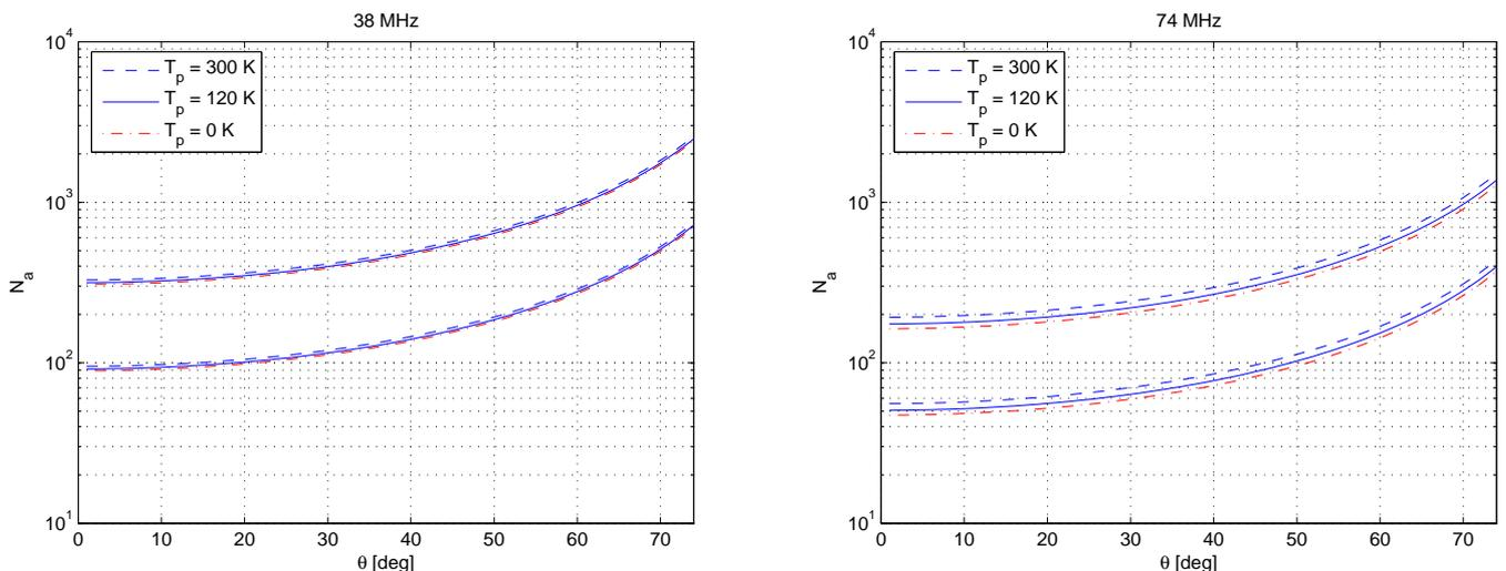
Fig. 5. Required number of dual-polarization antennas per station ( $N_a$ ) for  $N_S = 53$  with  $L_B = 400$  km. *Left:* 38 MHz, *Right:* 74 MHz. The upper set of curves assume  $N_{cal}^{VLA} = 10$  and  $r_{np} = 0.5$  whereas the lower set of curves assume  $N_{cal}^{VLA} = 4$  and  $r_{np} = 1$ . The right edge of each plot corresponds to upper culmination of the Galactic Center as seen from New Mexico.
