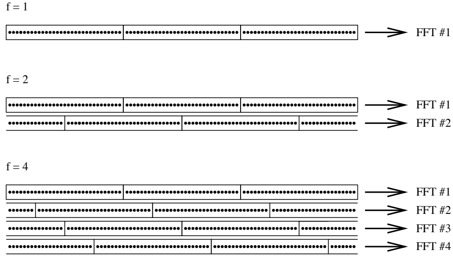
Figure 4–10. Cases of overlapped segmentation for N = 32 and f = \{1, 2, 4\} .
