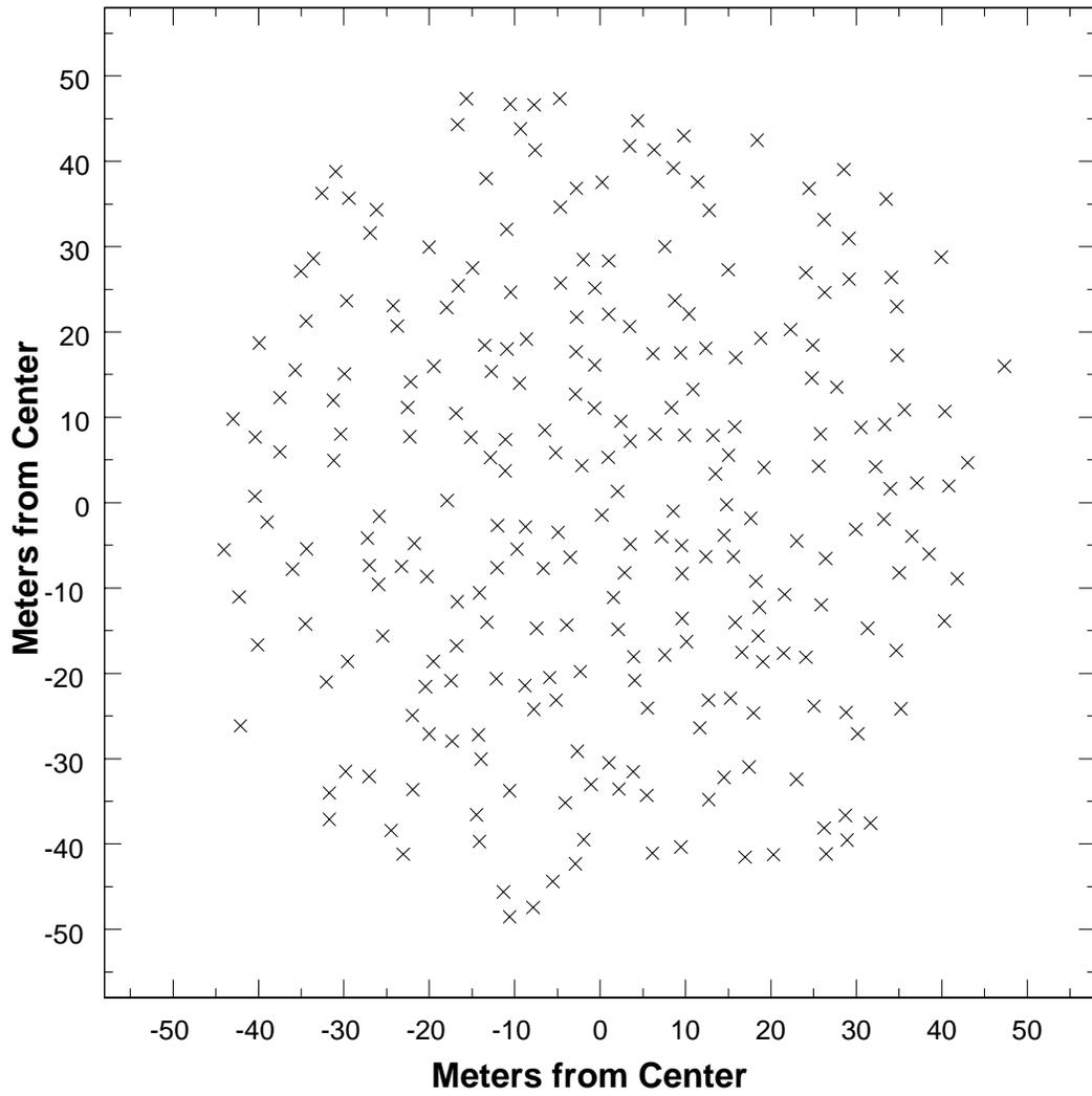
Figure 3: Station configuration after being optimized for sidelobe suppression with the constraint of a 2.0 meter minimum spacing between dipoles.
