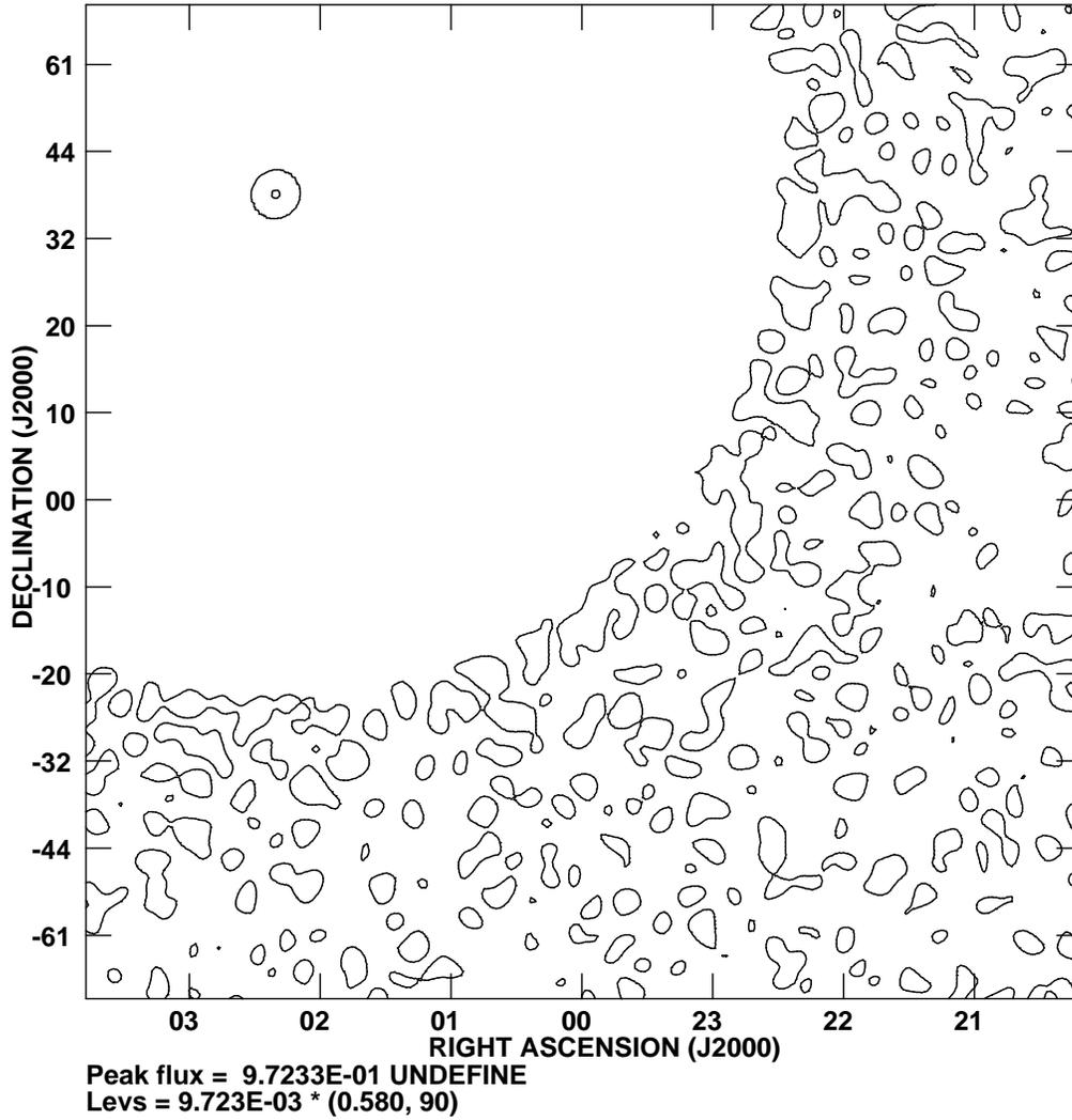
Figure 5: The two dimensional beam pattern phased towards  $|z_0| = 60^\circ$ ,  $|az_0| = 45^\circ$ . The same configuration used here as for the plot at the figure 4. Equation (1) is used to calculate the beam pattern. It is seen that this plot coincides with the beam pattern of the figure 4 but shifted from the center ( $z=0$ ) to  $|z_0| = 60^\circ$ ,  $|az_0| = 45^\circ$ .
