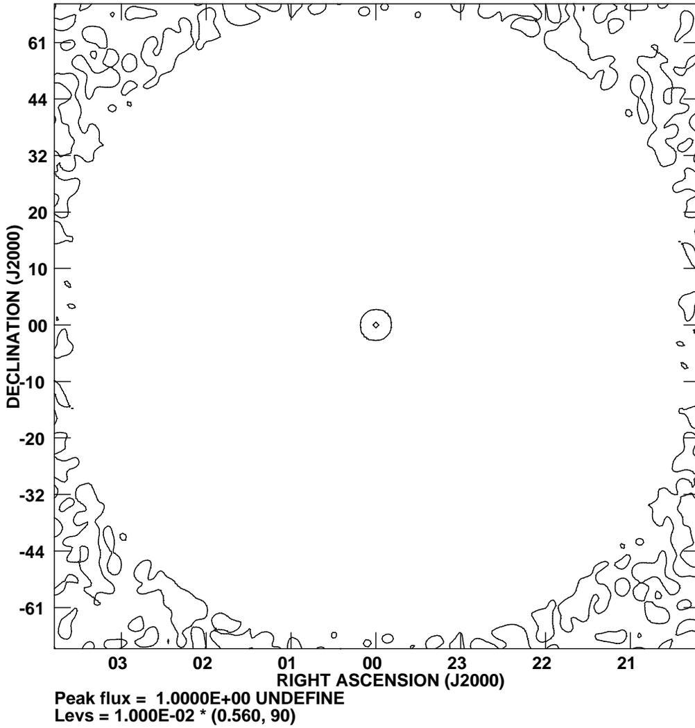
Figure 4: The two dimensional beam pattern created as a result of the optimization of the array with 256 antennas located inside of the circle 110 m diameter with minimum spacing 2 meters. The sky area of optimization is the whole semisphere  $|z| \leq 90^\circ, |\sin(z)| < 1$ . The polar coordinate at the plane corresponds to the radius equaled  $|\sin(z)|$ . The side lobes are less than 0.0056 (22.5dB) inside of the circle  $|z| < 90^\circ, |\sin(z)| < 1$
