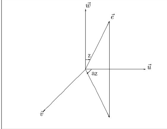
Figure 1: Coordinate system of the antenna station. The array antennas are located in the  $u - v$  plane. The  $w$ -axis is perpendicular to the array plane. The angle  $z$  is the angle between the  $w$ -axis and the given direction on the sky. The angle  $az$  is the azimuth of the given direction on the sky at the array plane.
