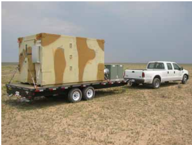
Figure 1. Shelter arriving at the LWDA site. AC unit is at the front of the trailer.
