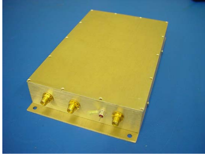
Fig. 3 Final design of LWDA receiver enclosure.
