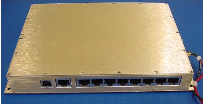
Fig. 1. Final design of LWDA adder board enclosure.
