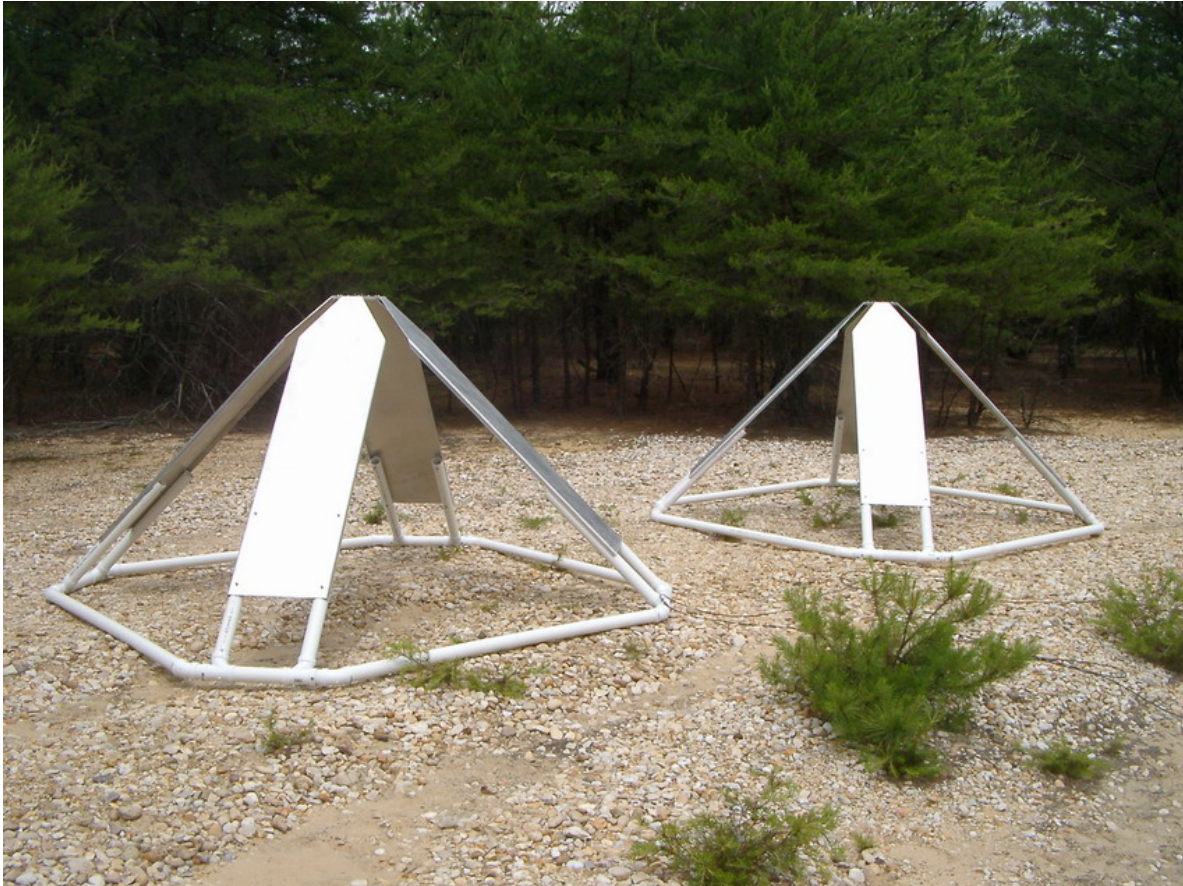
Figure 1. Two of the large blade dipoles and pyramidal supports used for cross-coupling measurements at the GSFC Observatory.
