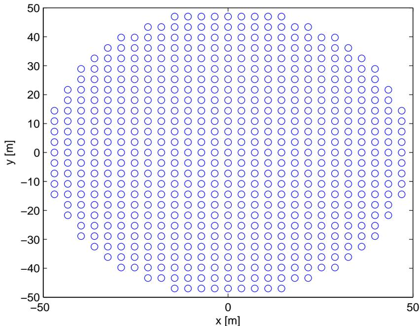
Figure 2: Compact array geometry. 593 stands, consisting of 593 co-polarized dipoles and no cross-polarized dipoles.
