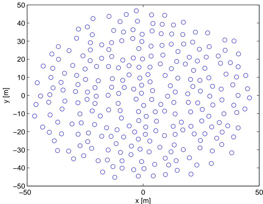
Figure 1: Sparse array geometry. 256 stands, consisting of 256 co-polarized dipoles and no cross-polarized dipoles.
