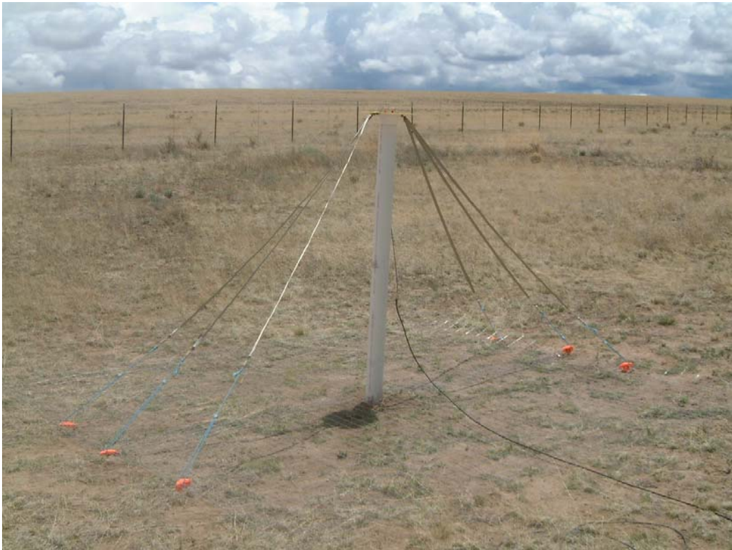
Fig. 4. The fork antenna on the 10'x10' ground screen.
