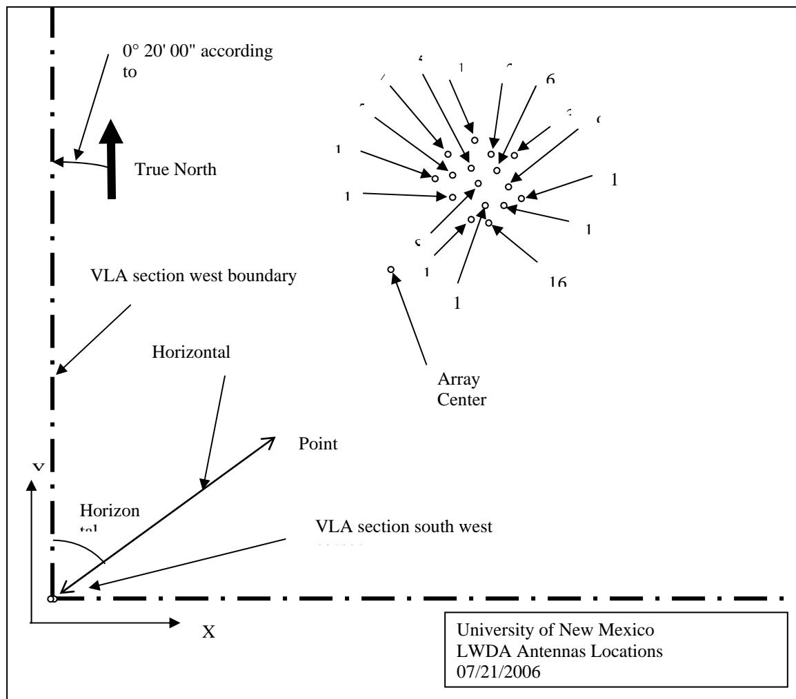
The reference point “VLA section south west” is taken as the “center” of the LWDA array. This point has ECI vector components  $S_X = -1602196.60$  meters,  $S_Y = -5042313.47$  meters, and  $S_Z = 3553971.51$  meters. In geodetic coordinates, this position transforms to 252.372 degrees east longitude, to 34.069 degrees north latitude, and to 2127 meters of local elevation.
