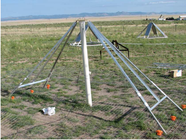
Fig. 4.— A photograph a single-polarization tied fork antenna prototype.
