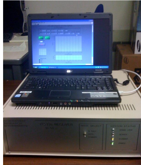
Figure 3: TBB Patch Antenna and Receiver. A patch antenna (left panel) used to observe the TBB signal is shown with its base support. The antenna is approximately 1-meter square. The assembly was broken-down for shipping and re-assembled at the VLA. The TBB receiver and accompanying laptop computer are shown in the right panel. The system requires 110 VAC and requires connection to the antenna via three coaxial cables (one for each frequency).
