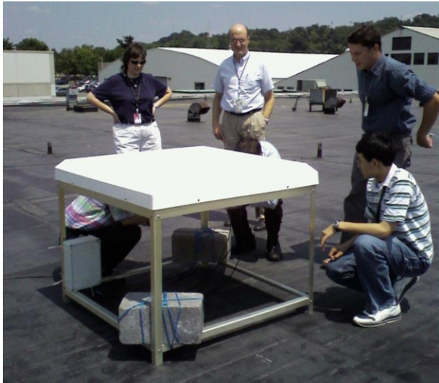
Figure 3: TBB Patch Antenna and Receiver. A patch antenna (left panel) used to observe the TBB signal is shown with its base support. The antenna is approximately 1-meter square. The assembly was broken-down for shipping and re-assembled at the VLA. The TBB receiver and accompanying laptop computer are shown in the right panel. The system requires 110 VAC and requires connection to the antenna via three coaxial cables (one for each frequency).
